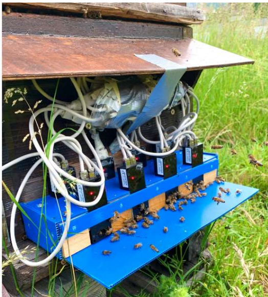
Figure S3: RFID system installed at the entrance of a honeybee colony.
