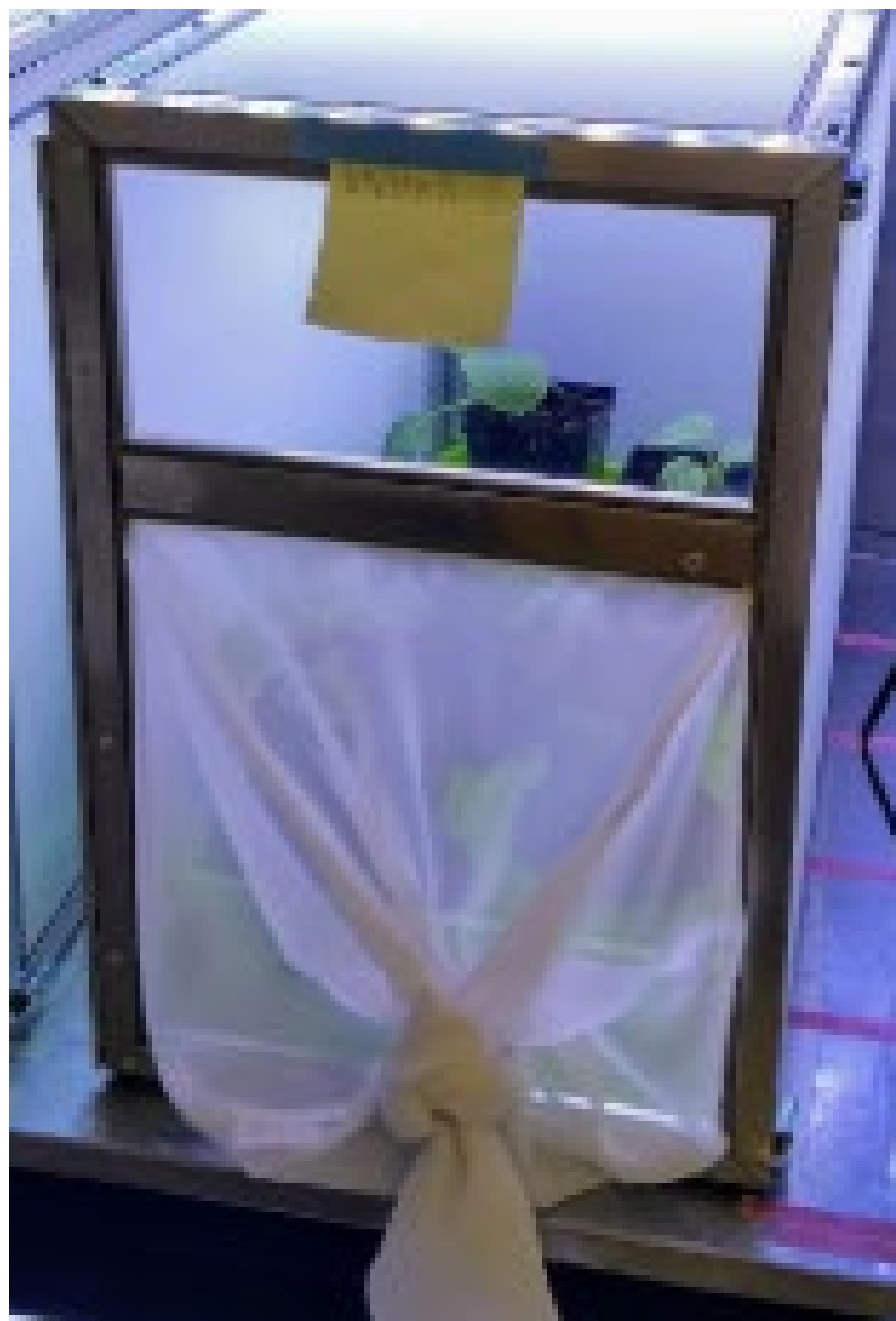
Fig. S1.6: Screen cage with plant flat to provide biocontainment of whiteflies. Cage used to house our potted whitefly colony as well as carry out quantitative proliferation studies as used for back-calculation of viability of a whitefly inoculation.
