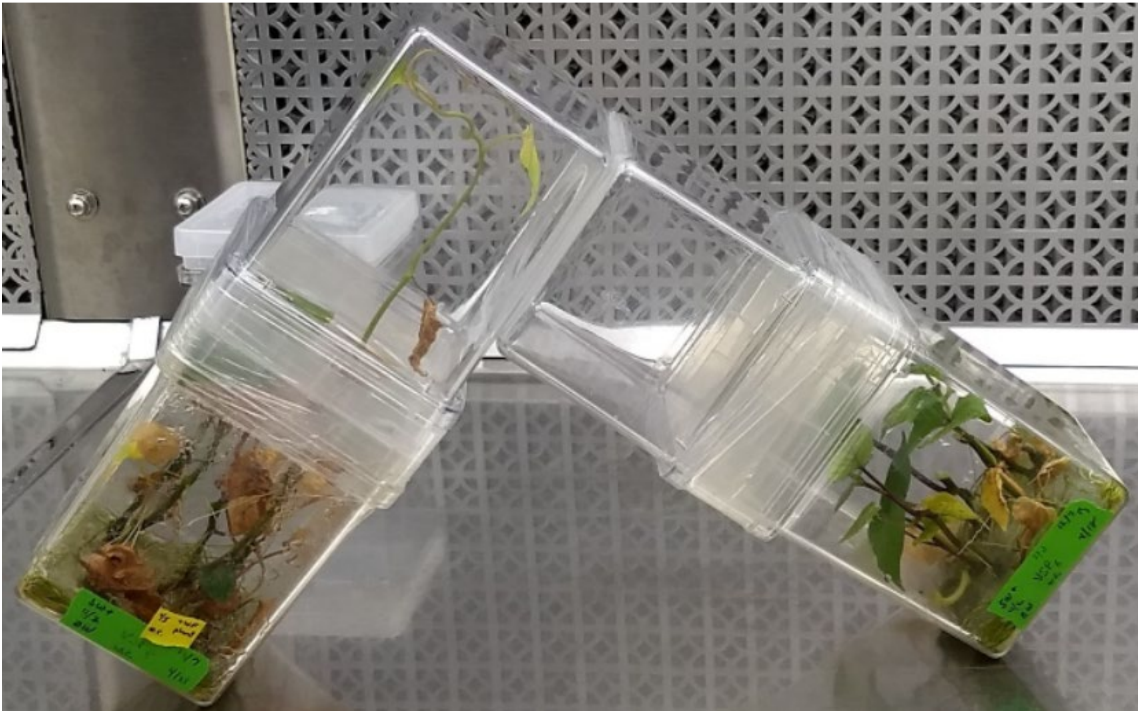
Fig. S1.1: Whitefly plant tissue culture L-Shaped axenic transfer device. Early transfer prototype created by connecting two GA7 couplers together with a hole. The L-shape allows for fresh plants to be swapped in below easily.
