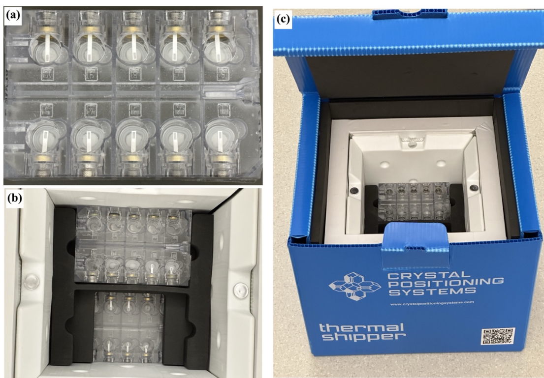
Figure S3. (a) Photograph of AFD-X chips loaded with protein crystals inside the SSRL crystallization plate for safe transport. (b) Multiple loaded plates stacked into the thermal shipper box. (c) Overview image of the thermal shipper box containing the SSRL plates.
