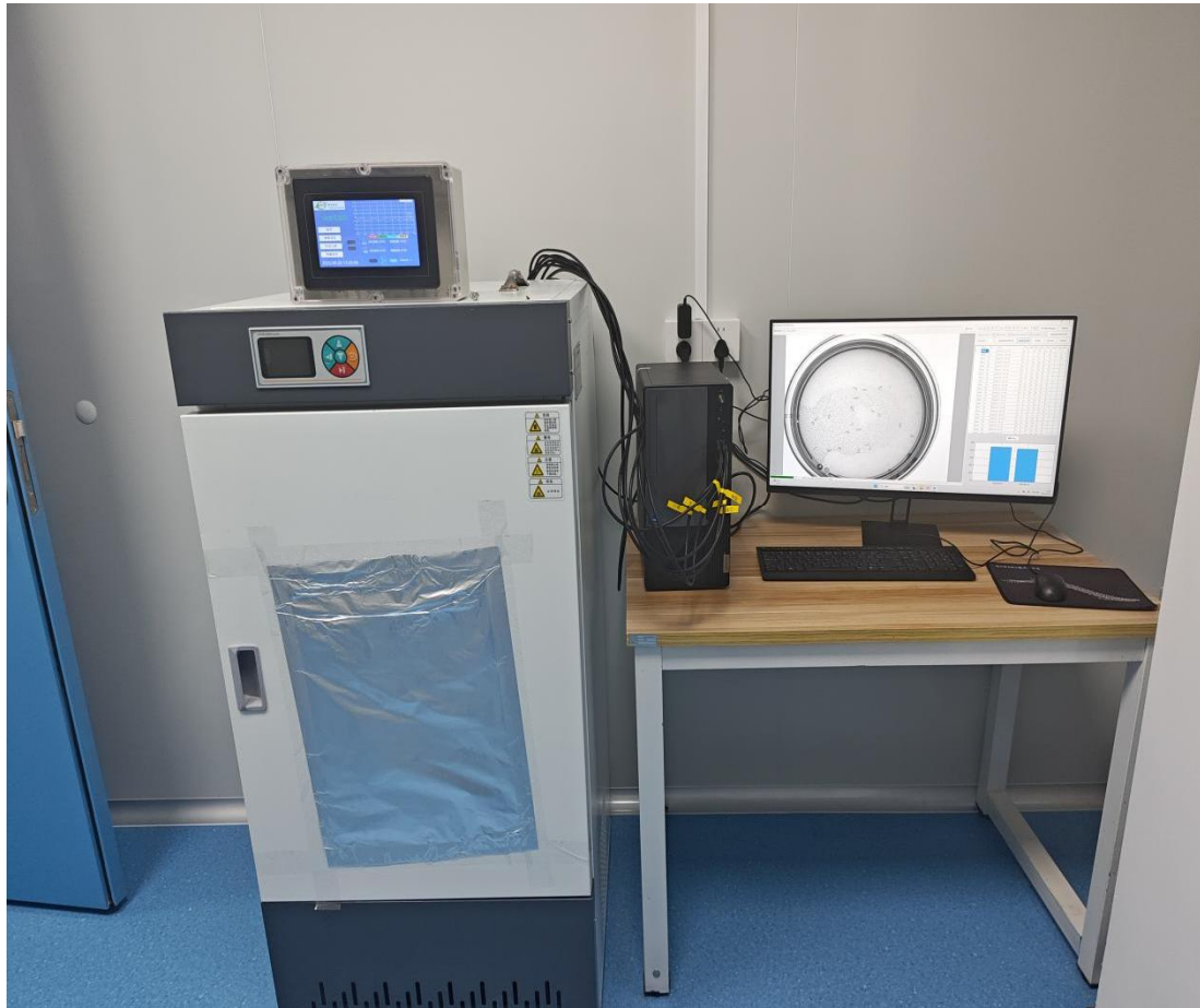
Figure S1. Physical diagram of the incubator and computer. The incubator (left) was purchased commercially and served as the base for subsequent modifications (e.g., circuit adjustment, fan airflow redirection, and lighting replacement), providing a stable culture environment for C. elegans . The host computer (right) runs the data acquisition software developed based on C# and .NET framework, connecting to industrial cameras and the incubator's serial port via USB interfaces to realize automated imaging control and environmental parameter regulation.
