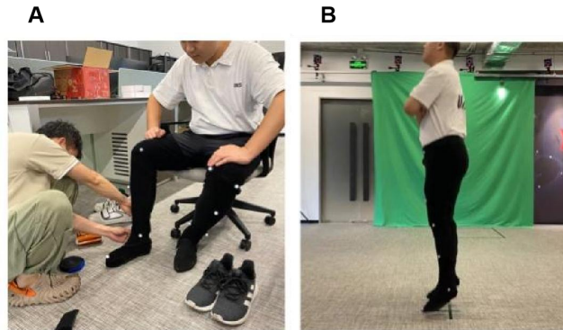
Figure 3. Kinematic data measurement: (A) Preparation for motion capture. (B) Kinematic data collection during the jumping process.
