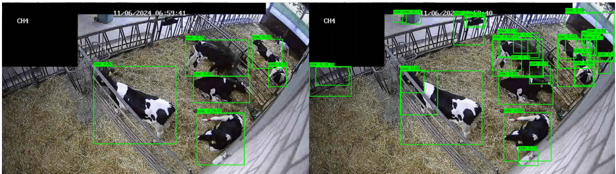
Figure S2. Bounding boxes overlaid with predictions from YOLOv12 (left) showing successful detections of cows within the frame, and OWLv2 3 detection output (right) demonstrating false positive generation at default confidence settings.
