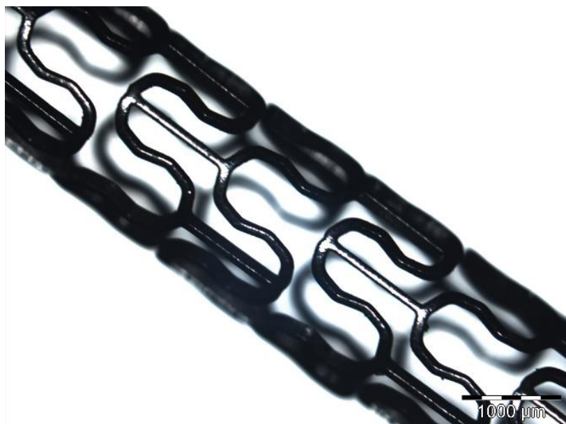
Supplementary Figure S17 | Optical microscope image of the X-rayed coronary stent. The scale bar corresponds to a length of 1000 \mu\text{m} . The stent with 2 mm diameter has a rectangular metallic mesh with sizes of 100 \mu\text{m} \times 200 \mu\text{m} .
