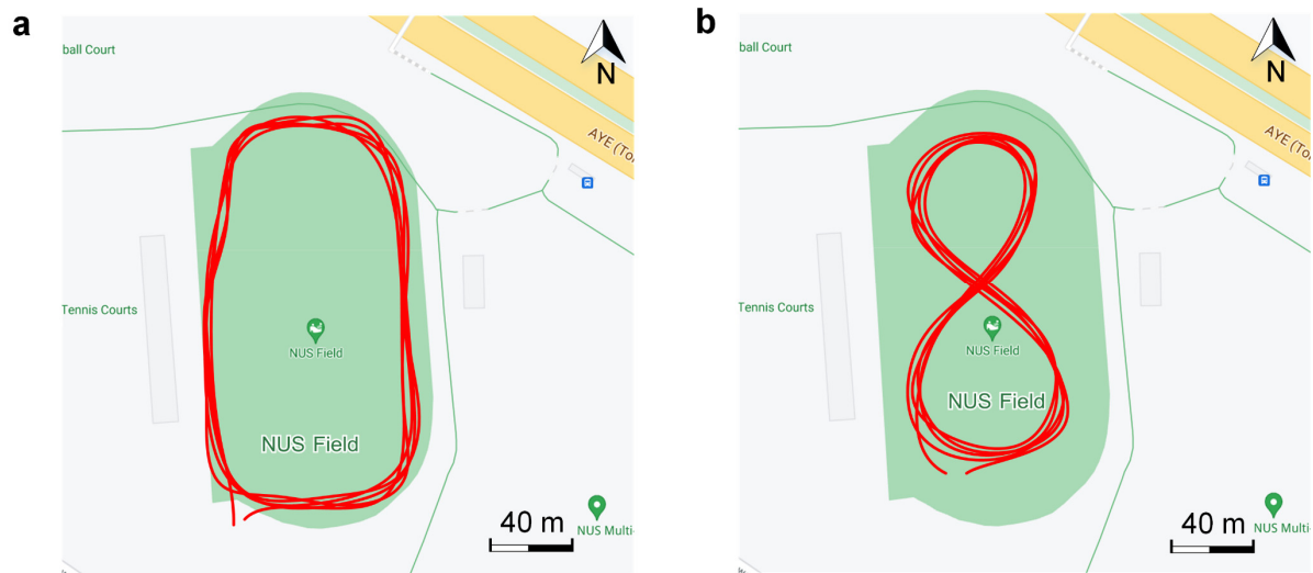
Extended Data Fig. 13 | Demonstration of wheelchair navigation. a and b , Flexibility and accuracy test for wheelchair navigation over 1.6 km around a standard 400-m running track. Circular and figure-8-shaped wheelchair motion trajectories were recorded using the global positioning system (GPS) after five tests. Scale bar: 40 m.
