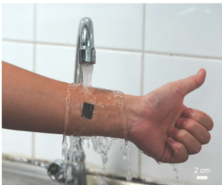
Supplementary Fig. 28: Optical image of 1 \mu\text{m} -thick PUNF-PDMS-Au-pDAM electrode attached onto an arm that was durable against heavy water washing.
