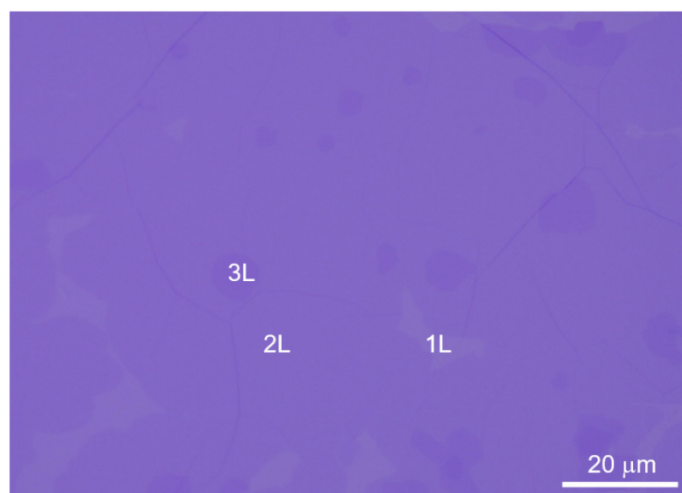
Supplementary Fig. 3. UV tape transfer of bilayer graphene from Cu-Ni film. The BLG grown on a Cu-Ni(111)/sapphire substrate was transferred on a SiO 2 /Si substrate using the UV tape. The surface of the transferred BLG is very clean without apparent breakages, indicating that the tape transfer is not limited to monolayer graphene nor Cu catalyst.
