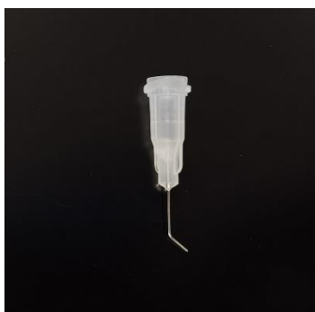
Figure S16. A curve needle with a bending angle of 45 °.
