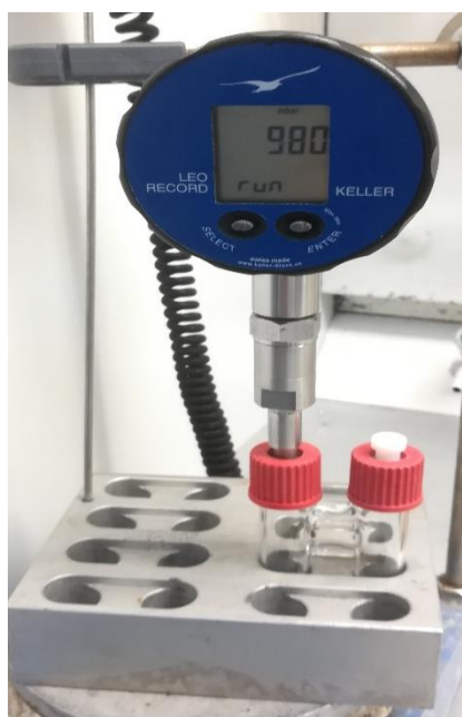
Supplementary Figure 3. Two-chamber reactor fitted with a manometer (chamber A)
