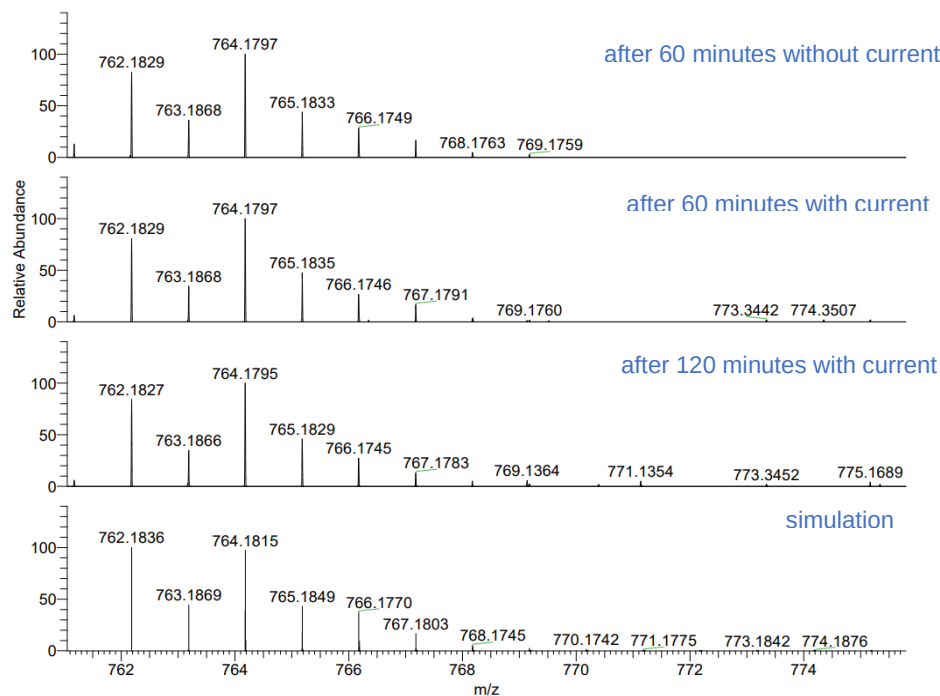
Supplementary Figure 15. HR-ESI-mass spectrometric monitoring of the enantioselective electrochemical nickel-catalyzed C–H activation. m/z calculated for [\text{C}_{41}\text{H}_{43}\text{BrN}_3\text{NiO}_3]^+ = 762.1836 .
