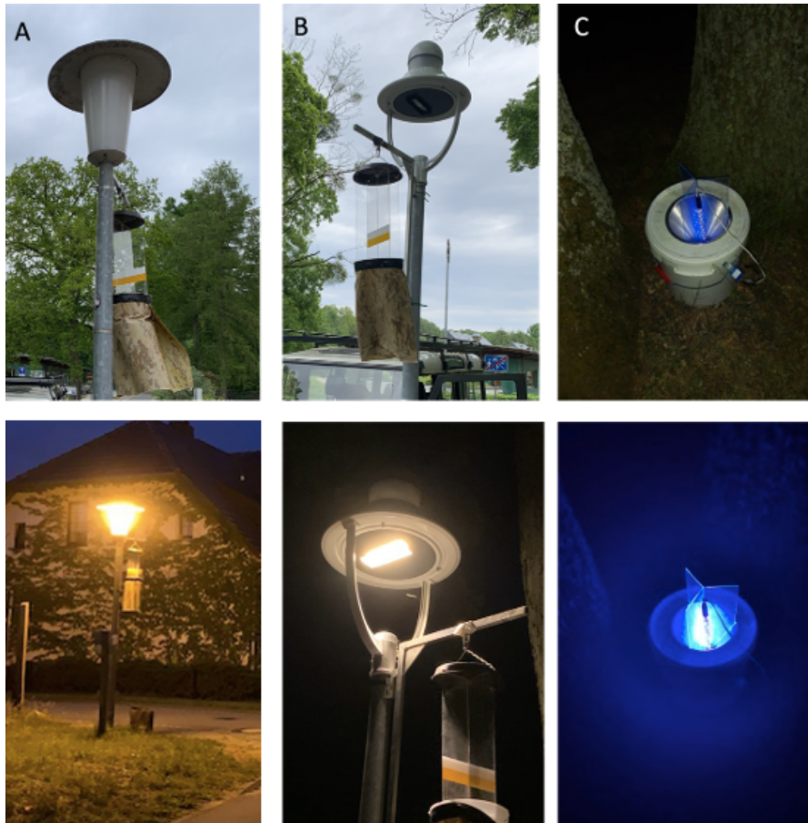
Figure S4: Luminaire and trap types. Top: Map shows locations of individual road lights/ UV traps. Bottom: HPS column luminaire with flight interception trap (3.3m height) (A), tailored and shielded luminaire with flight interception trap (3.3m height) (B) and UV traps on
