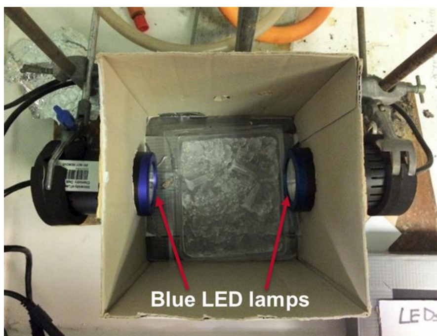
Supplementary Figure 14: Photolabelling set-up: two Kessil H150W-BLUE LED lamps facing each other, parallel to base of the box containing the samples in Eppendorf tubes.
