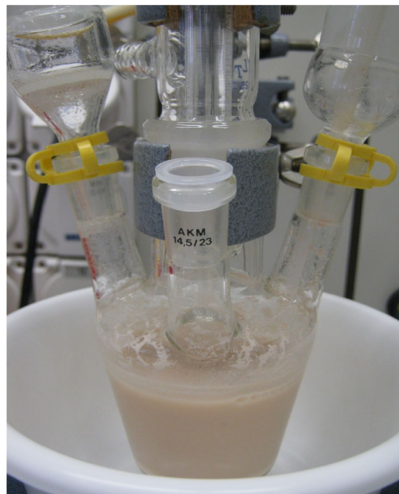
Supplementary Figure 12. 100 mL-scale reaction set up for reduction of 1a by variant M6 in the iPrOH-based recycling system. a Start time. b After 4 hours. The reaction vessel contained 1a (10 g, 0.03 mol, 1 eq), water (39 mL), 1 M potassium phosphate buffer pH 7.2 (10 mL), 0.1 M \text{MgCl}_2 \cdot 6\text{H}_2\text{O} (2 mL), iPrOH (8 mL), \text{NADP}^+ (100 mg, 0.004 eq, s/c = 100, previously dissolved in 1 mL), and M6 lyophilized lysate (2 g, s/e = 5, previously dissolved in 30 mL water). The reaction was run at 23 °C for 30 h.
