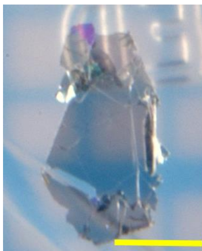
Supplementary Figure 1. Optical image of typical flake-like h-BN sample. Scale bar is 1 mm.
