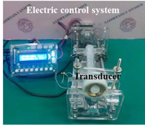
Fig.S8 Photograph of the microinjection pump system.
