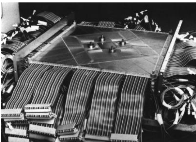
Figure 1 NA14 Detector Stack. Each plane has a single-sided 1000 strip 5cm×5cm silicon detector at its centre. Reproduced from Ref. [2]
