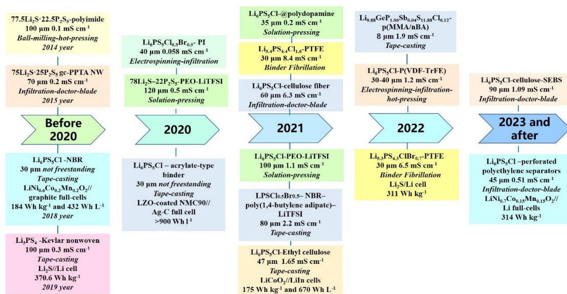
Fig. 6 A brief chronology of development of some important events in sulfide-based composite solid electrolyte films for all-solid-state batteries
