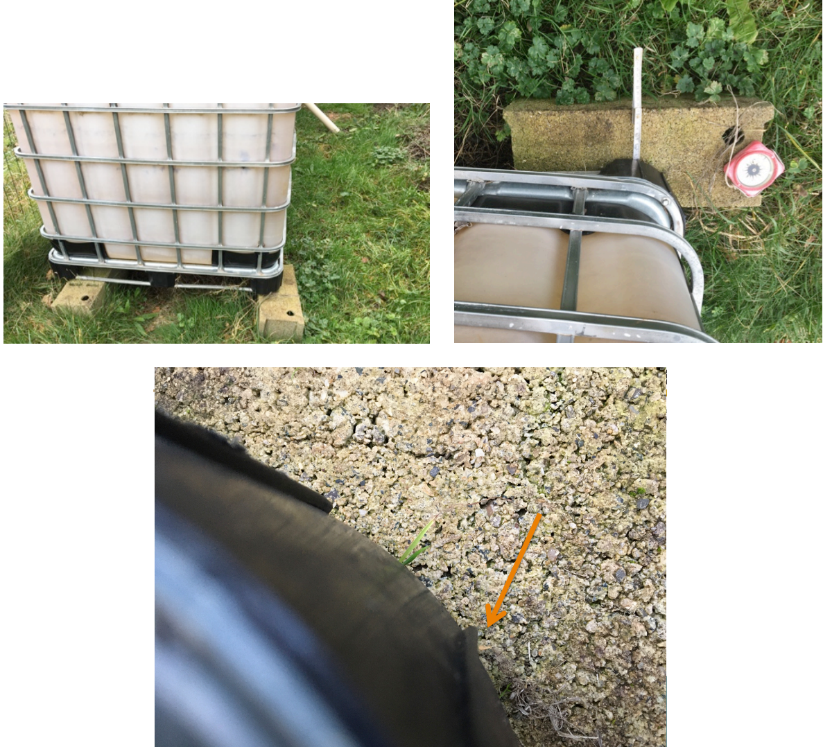
Figure S6.8.: DT, displaced water-tank site. Three displaced water tanks (1 ton each). (top left) full view of one tank; (top right and bottom) zoom on the distance in between former tank location (ageing tank imprint on the concrete-stone) and the post earthquake location that points on a 5 cm displacement without friction evidence.
