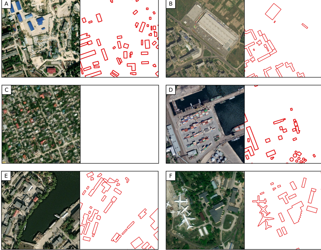
Fig. S3: Quality issues of existing building footprints. All images cover 500 \times 500 \text{ m}^2 and are displayed alongside the corresponding building footprints sourced from Overture Maps. Only buildings larger than 50 \text{ m}^2 are depicted. (A) Outdated buildings in Sevastopol. (B) Absent shopping mall near Chernihiv. (C) Missing footprints in Kherson. (D) Containers in Odessa. (E) Boats in Zaporizhzhia. (F) Antonov International Airport, Hostomel. Satellite images were obtained from ESRI/Maxar Technologies (A and C), Bing/Maxar Technologies (B, E, and F), and Google/Maxar Technologies (D).
