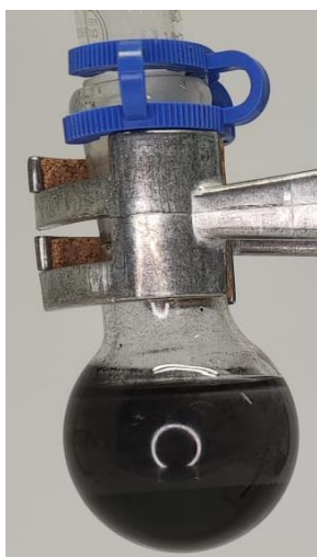
Figure S114. [P_{4441}][HSO_4] in acetonitrile with activated charcoal.
