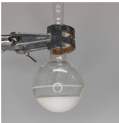
Figure S121. White solid precipitated in the crude mixture after 24-h stirring at room temperature.
