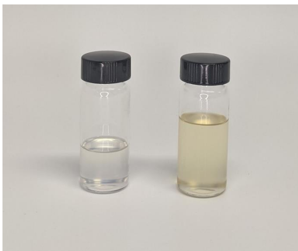
Figure S8. 1-bromobutane (left) and sulfuric acid phase (right) collected in vials.
