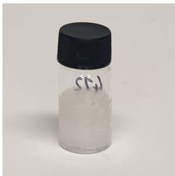
Figure S84. Dried [P_{4441}][OAc] (mixture of phosphine isomers)
