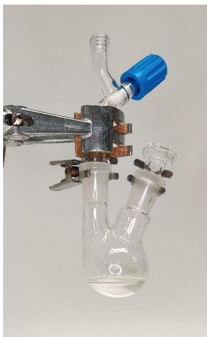
Figure S152. Homogeneous reaction mixture after addition of methyl triflate and stirring.
