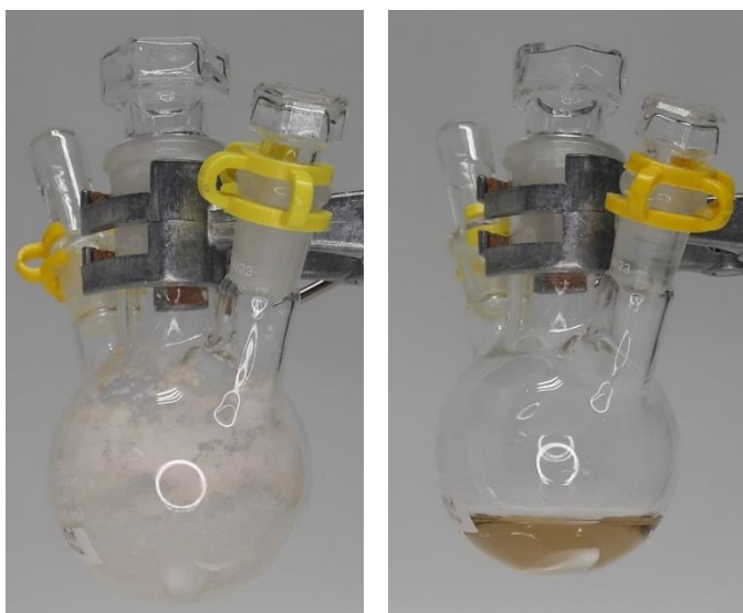
Figure S38. [C_4Py]Br after one recrystallisation: solid (left), dissolved in acetonitrile (right). The solid powder looks off-white, but the solution is yellow.
