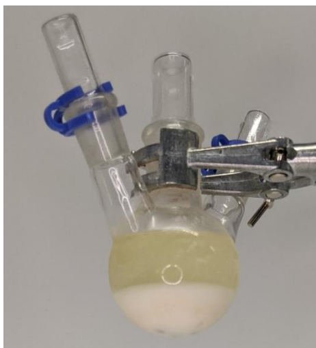
Figure S49. First recrystallisation of [C_4Py]Br .
