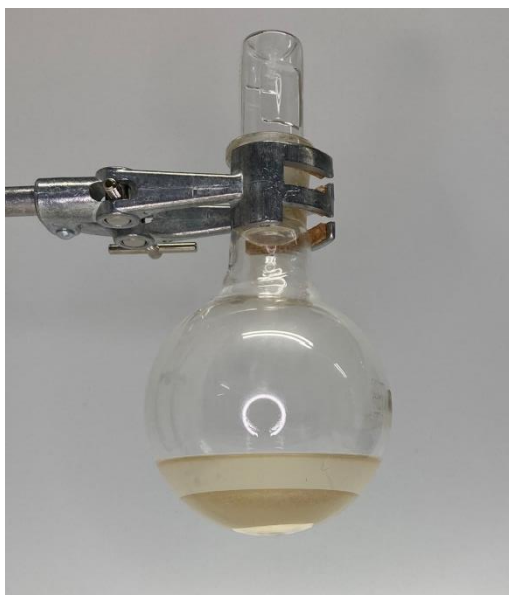
Figure S20. Crude reaction mixture after 1 day. Top phase contains ethyl acetate and unreacted starting materials, while bottom phase contains [C_4C_4im]Br .
