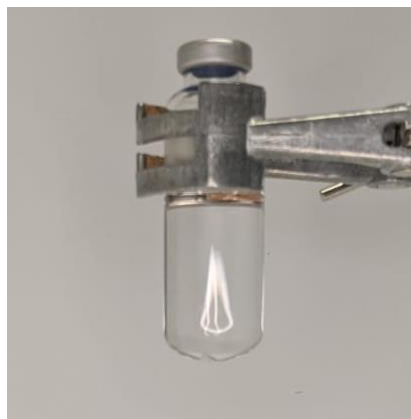
Figure S56. Thick-walled vial with sealed cap, suitable for the microwave reactor.
