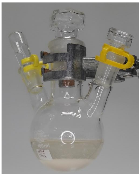
Figure S39. Second recrystallisation of [C_4Py]Br .
