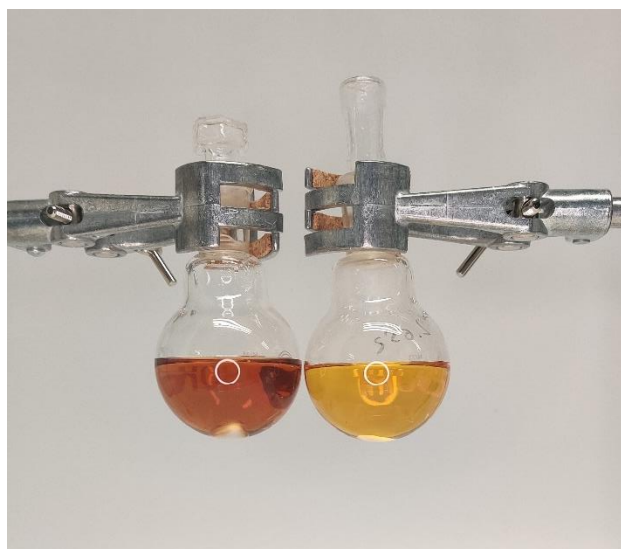
Figure S97. [\text{C}_4\text{C}_4\text{im}][\text{OAc}] with HBr (left) and with HCl (right).
