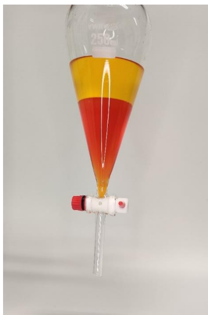
Figure S94. First ether wash of the reaction mixture. Top layer: ether phase, bottom layer: IL phase.
