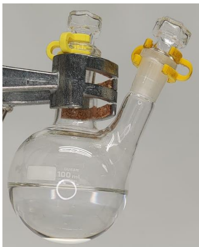
Figure S106. Two-layer system indicating the formation of [P_{4441}][C_1SO_4] .
