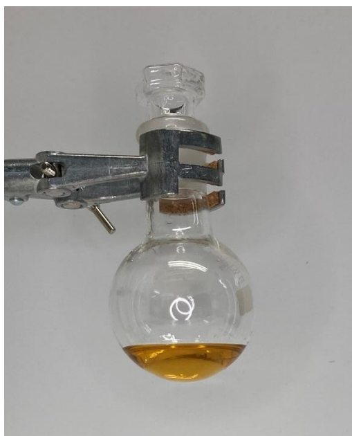
Figure S21. Crude [C 4 C 4 im]Br before purification.
