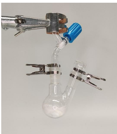
Figure S135. Product after drying in high vacuum.
