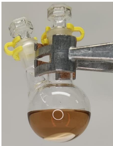
Figure S103. Dimethyl sulfate, as received from the bottle. Brown colouration indicates decomposition.
