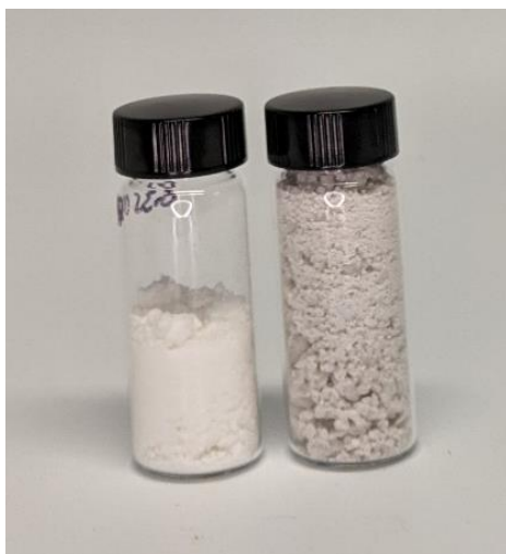
Figure S61. Comparison between the product of controlled (left) and uncontrolled (right) MW-assisted reaction.
