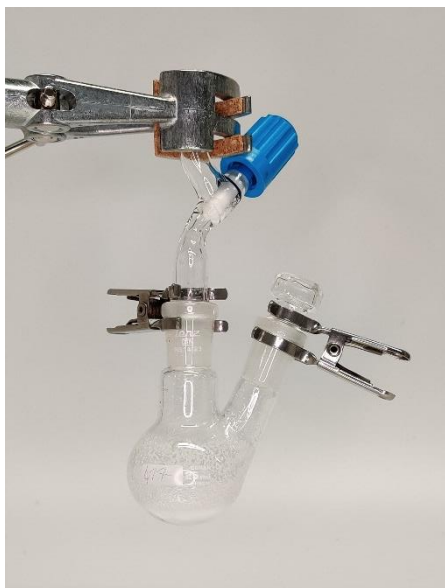
Figure S134. Reaction mixture after the addition of methyl triflate and stirring for 30 minutes.
