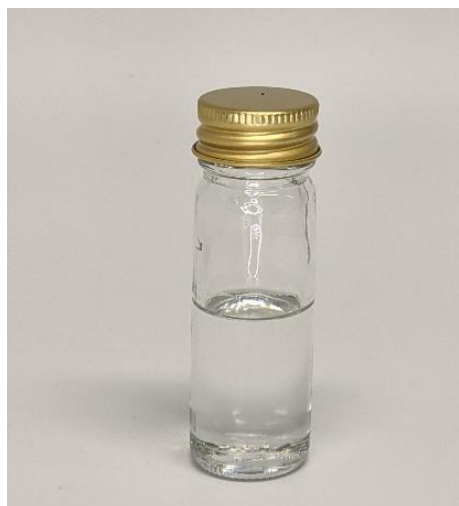
Figure S47. Thick-walled reaction vial. Suitable for sonication probe.
