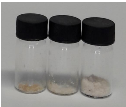
Figure S42. Comparison of [C_4Py]Br before recrystallising (left), after one recrystallisation (middle) and after two recrystallisations (right).
