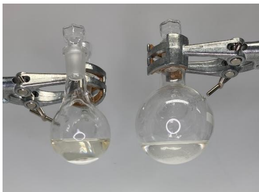
Figure S27. Crude reaction mixtures after 1 day of stirring. Left is the reaction using acetonitrile (homogeneous solution), while right is the reaction using ethyl acetate (white precipitate starts forming).
