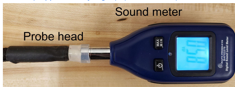
Supplementary Figure 5: Sound level calibration. A sound meter (BAFX 3370, Digital Sound Level Meter, $18) is used to calibrate the sound level produced by our system.
