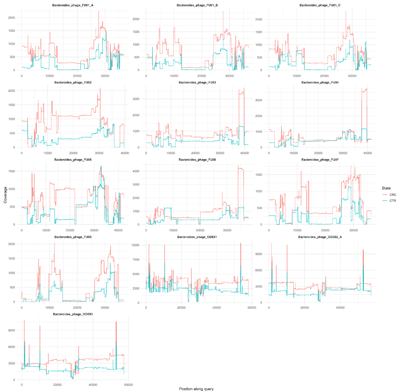
30 Figure S5. Weighed coverage of the Bacteroides phage genomes from the metagenomic 31 cohort screening on patients with colorectal cancer (CRC, red, N = 434) and controls 32 (CTR, blue, N = 443). Assembled metagenomic contigs were screened with MASH and 33 BLASTN to identify matching sequence fragments as described in methods. Weighed 34 coverage is given by the accumulated coverage of all high quality BLASTN matches 35 (bitscore >50).
