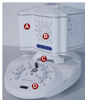
Fig. S4. Scheme and photograph of the ThalesNano PhotoCube™ reactor.
