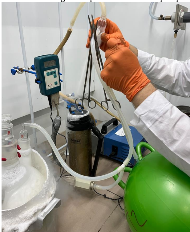
Disconnecting the trap of the membrane pump
