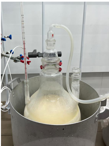
Stable operating mode – \sim -10\text{ }^{\circ}\text{C} temperature reaction mixture
