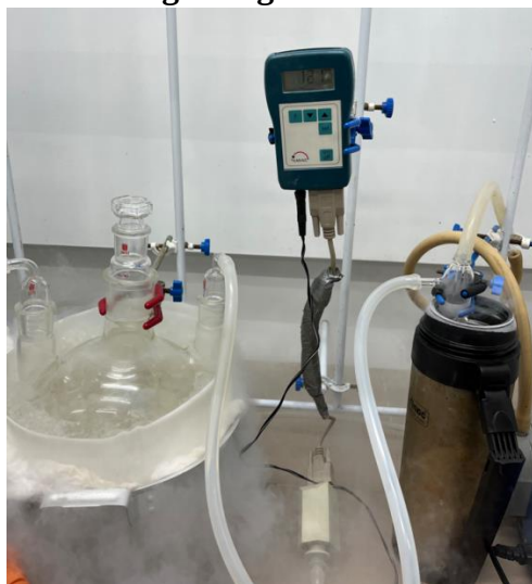
Entering the mode of stable distillation of BCP
