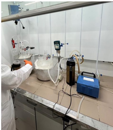
Stable operating mode – \sim -10\text{ }^{\circ}\text{C} temperature reaction mixture
