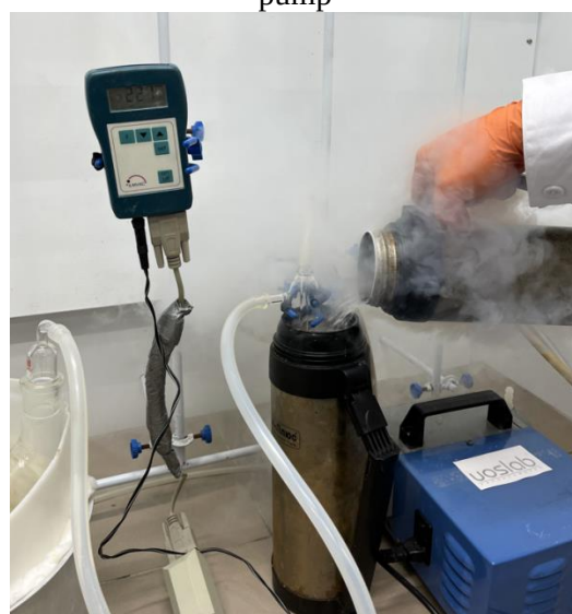
Cooling of the protection trap of the diaphragm pump
