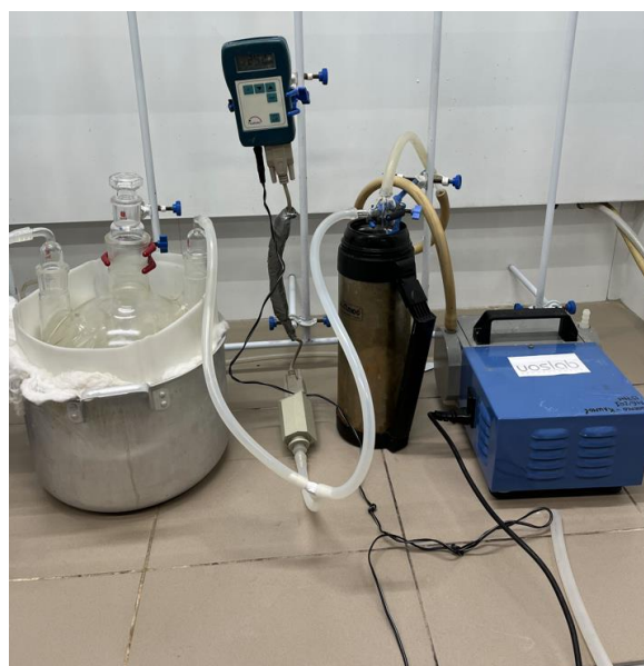
Cooling of the protection trap of the diaphragm pump
