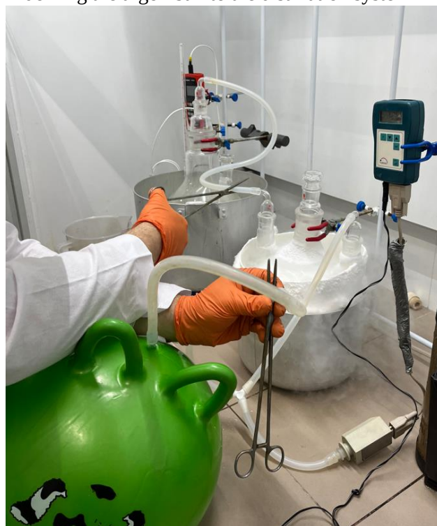
Joining the argon ball to the distillation system
