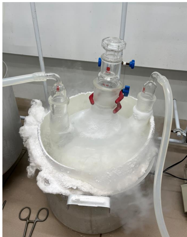
Joining the argon ball to the distillation system
