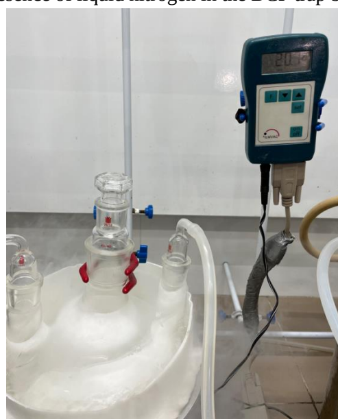
Stable operating mode after adding warm water to the bath – \sim -10\text{ }^{\circ}\text{C} temperature reaction mixture. Until the end of distillation:
