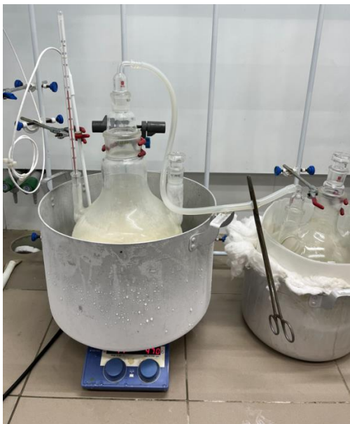
Cooling of the BCP trap (4 L three-necked reactor)
