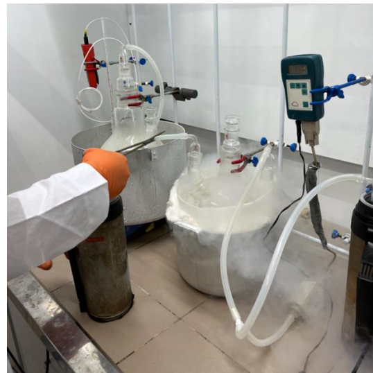
Entering the mode of stable distillation of BCP
