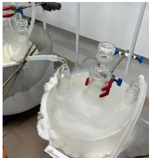
Stable operating mode – \sim 20\text{ mbar} pressure of the system. Until the end of distillation keep the presence of liquid nitrogen in the BCP trap bath.
