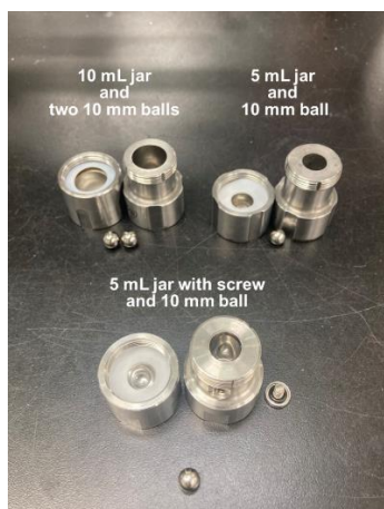
Figure S2. Stainless jar (10 mL and 5 mL) and balls (10 mm) used in this study.
