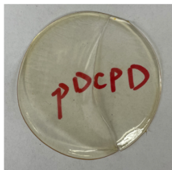
casted film from unfunctionalized oligo-DCPD
