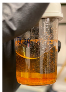
insoluble crosslinked solid forms immediately
