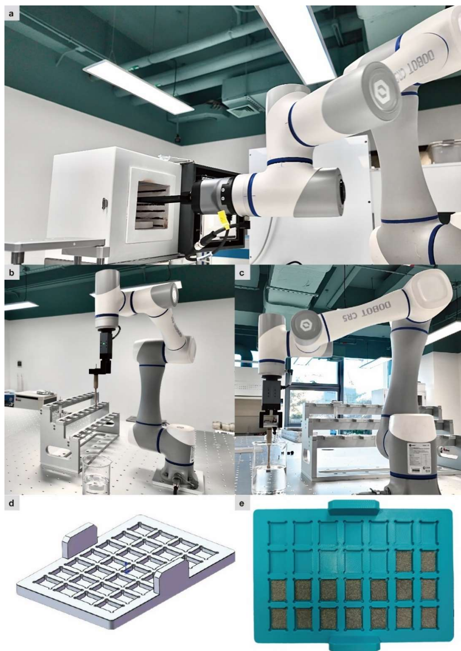
Fig. S32 Photograph and demonstration of the 6-axis robotic arm in high-throughput experimental workflows. a , The robotic arm showcasing its adaptability for tasks such as sample assembly, pick-and-place operations, and furnace loading/unloading. b , The robotic arm holding \text{CeO}_2\text{@NF} (nickel foam) and featuring a custom-fabricated metallic electrode holder with a capacity for over 100 electrodes. c , The robotic arm immersing \text{CeO}_2\text{@NF} into a VC solution. d , 3D rendering of a sample stage designed for storing electrodes. e , Photograph of the actual sample stage.
