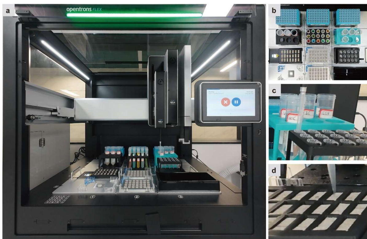
Fig. S33 A liquid handling robot completes the SAC loading process.
