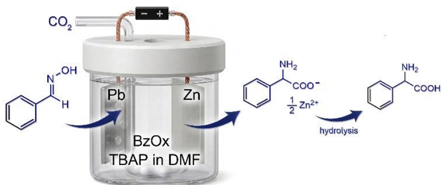
Figure R6 (new Figure 3a). Schematic illustration of electrochemical reductive carboxylation of BzOx with CO 2 .
