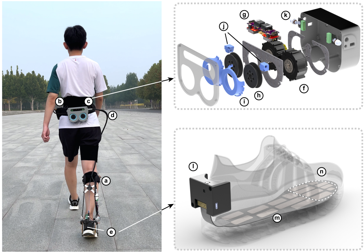
Supplementary Figure 2 | Photograph of outdoor walking with mobile ankle exoskeleton. The mobile unilateral ankle exoskeleton consisted of (a) a lightweight ankle exoskeleton end-effector worn on the right ankle; (b) a 4700-mA h portable lithium battery that allows for 3 hours of continuous assisted walking; (c) a waist actuation pack; (d) flexible Bowden and signal cables that connected the end-effector and the actuation system; (e) an arrayed pressure insole; the waist actuation pack comprised (f) two brushless DC geared motors; (g) an embedded control circuit board that implemented real-time closed-loop control and assistance optimization; (h) output pulleys driving the inner Bowden cables and protected by (i) the pulley covers; (j) two Bowden mounts that fixed the Bowden sheath; (k) two bridging boards connecting the signal cables. The pressure insole comprised (l) an acquisition unit and (m) a filmy insole containing 16 arrayed pressure sensors, with (n) the forefoot zone sensors used for outdoor ankle moment estimation.
