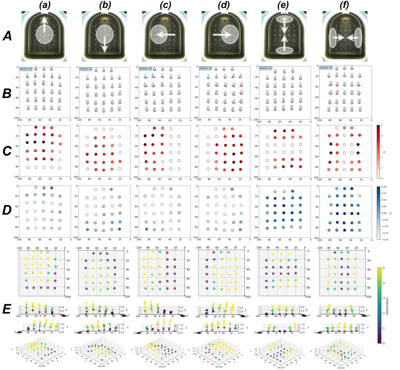
Fig. 1: In-sensor computing spatial contact response of PixelTac. A: Representative contact patterns, including four single-contact directions (a–d) and two opposing-contact configurations (e, f). B: Corresponding marker displacement vectors under each contact pattern. C: Marker displacement magnitude ( D_i ). D: Marker Gaussian density ( G_i ). E: Estimated contact deformation visualized from multiple viewing angles, with color indicating the deformation magnitude.
