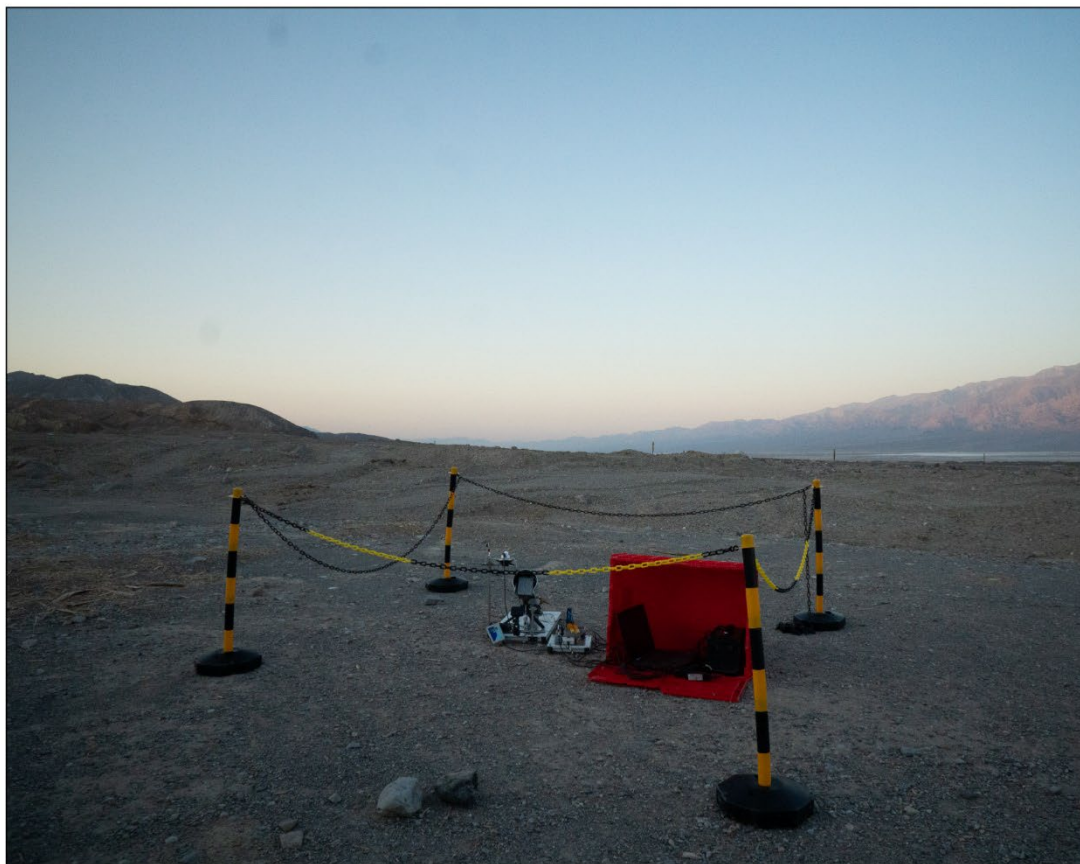
Supplementary Fig. 22. Photographs of the device test in the Furnace Creek ( 36.4506^{\circ} N, -116.8523^{\circ} W). (a) MOF cartridge during the night cycle of the August 23 2022 test. (b) Device at the end of the day cycle (after sun set). Red cargo box was used to protect the electrical devices from the direct exposure to sunlight.
