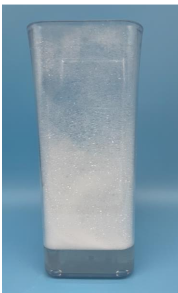
Fig. S2. Photo to visualize the vigorous foam formation of Buckeye AFFF at 1 to 100 dilution treated by EO without UV/S pretreatment. The EO flow cell was operated at 5 A to treat 200 mL diluted AFFF to showcase the foaming.
