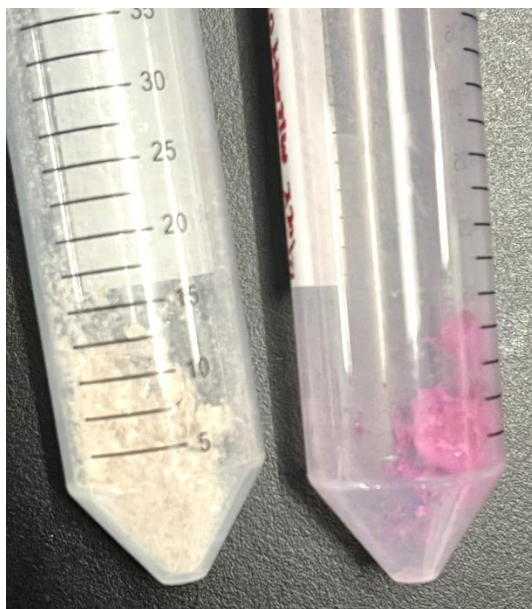
Supplementary Figure 3. Macroscopic photograph of poly(DMA-co-SBMA) ( Left ) and poly(DMA-co-SBMA-co-RhoB) ( Right ), with the pinkish color being attributed to the incorporation of RhoB within the copolymer.
