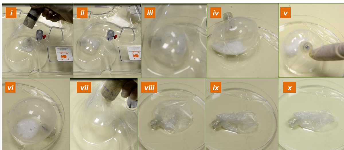
Fig. S8: Inflation and deflation for the balloon in simulated gastric acid environment; (i) Approach of the external magnet; (ii)-(iv) Inflation valve open, chemical reaction and CO 2 gas is created; (v) A few shakes are applied to stimulate the stomach motion; (vi) End of the reaction process; (vii) External magnet is introduced again; (viii)-(x) Deflation valve is opened and the balloon is completely deflated.
