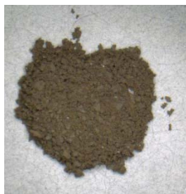
Figure S3. Photograph of the mixture of Si(com)-ba(w) and 5 wt% of graphite (200 mesh, 99.9995% graphite powder, Alfa Aesar).
