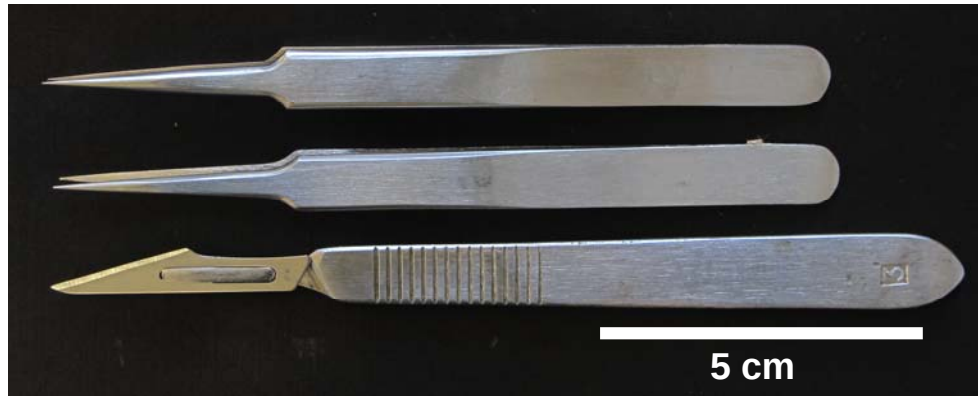
Figure S1. Forceps and scalpel used in crossing. Two pairs of fine tip forceps, e.g., HL-14 #5, www.buyincoins.com , and a straight-edge scalpel, e.g., scalpel blade handle 9303 #3, and scalpel blade 9311 #11, both from www.microscopesamerica.com , were used for keel petal incision, the removal of anthers from the unopened female flower bud and cross-pollination. Similar forceps and scalpels are available from other vendors. Bar=5cm.
