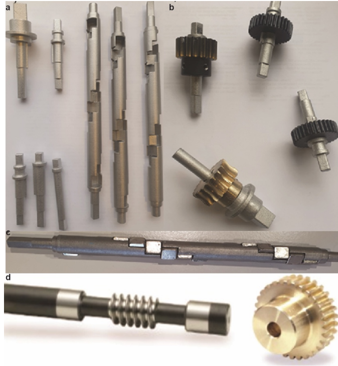
Fig. S8 | a , Pump axles (including the axles on which the magnets are installed, as well as the axles responsible for the maintenance and rotation of the gears. b , Assembling axles with pump spur gears. c , Installing 16 cubic magnets on the shaft. d , Worm gears
