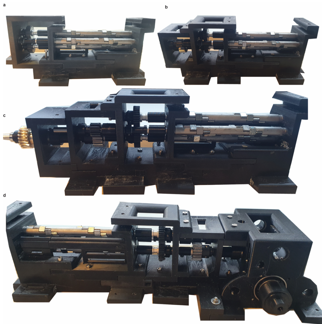
Fig. S12 | a , Positioning the shafts in the pump and adding two spur gears. b , Adding a spur gear for the shaft with twice the speed of the other shafts. c , Positioning of the central power axis system of the pump. d , Positioning of the gearbox in the electromotor.
