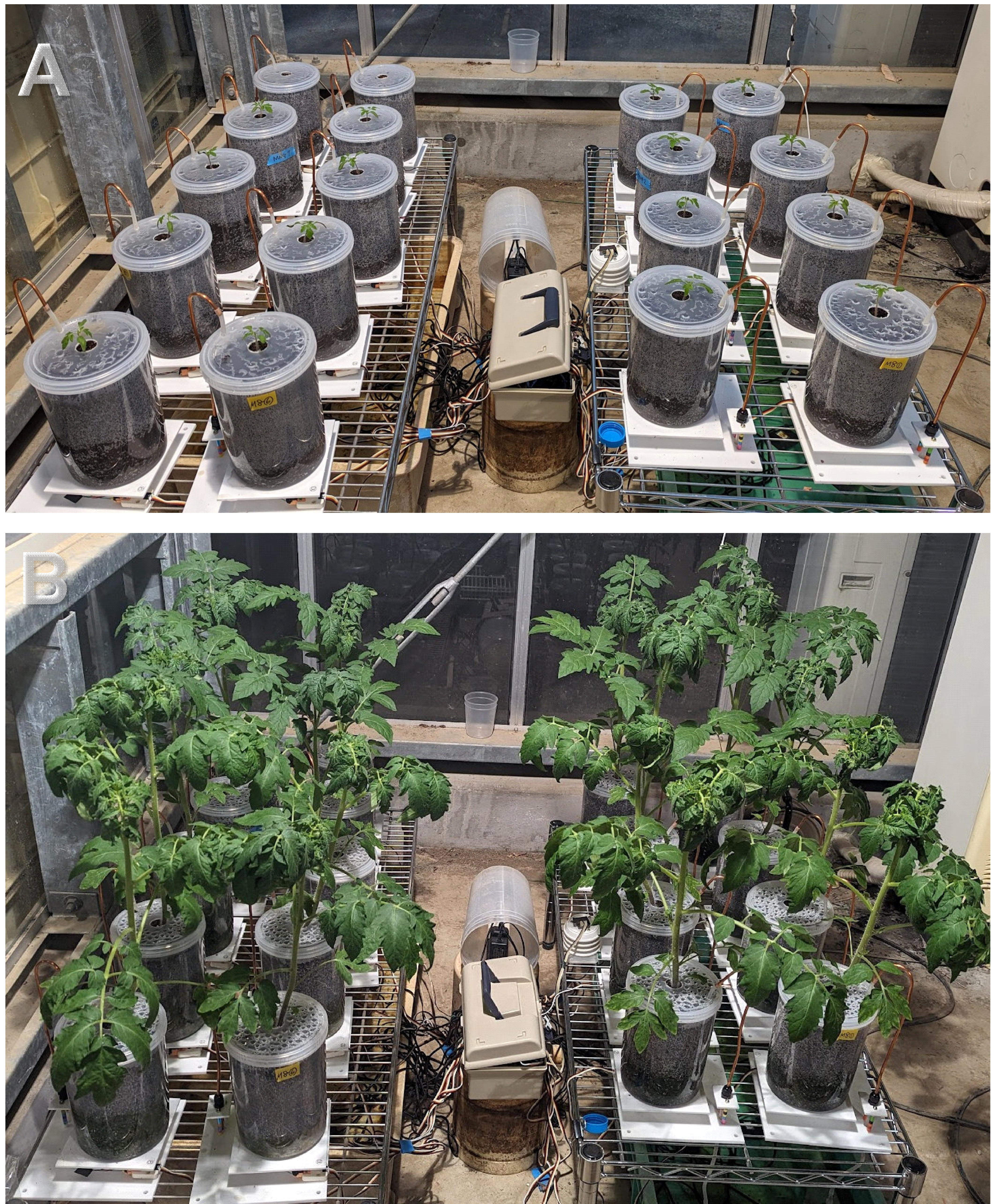
Fig. S1. A separate growth experiment conducted with the microcontroller-based water control system. 16 tomato plants were grown in lidded pots. (A) Just after transplanting and (B) 20 days after transplanting. Scales equipped with watering pipes are placed on the metal racks, with water tanks located under each rack. The microcontroller system is housed in the central plastic box.
