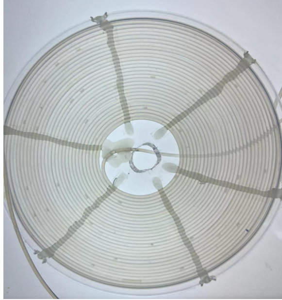
Figure S3. The generated droplets are introduced into Teflon tubes for incubation.
