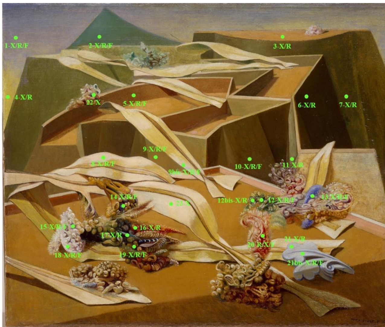
Figure S 2: Points analysed on the Garden airplane trap by the different techniques. X: XRF, R, Raman spectroscopy, F, ER-FTIR.
