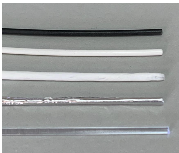
Figure S3. Different fiber coatings tested including from top to bottom black acrylic paint, white acrylic paint, teflon tape, aluminum foil and no coating.
