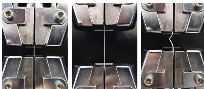
Figure S24. Photographs obtained during the tensile test. The samples were separated at the midpoint.
