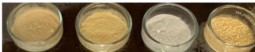
Supporting Figure S2: Photographic examples of polymers before and after 14 days of weathering in UV and cyclic temperature and humidity variations.
