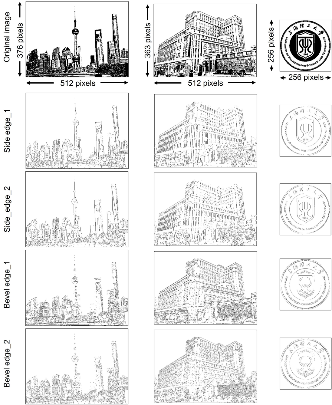
Supplementary Figure 16. Edge extraction results from various images processed by the four MI-DNNs, each with different target edge patterns. The grayscale of the images has been inverted for clearer observation.
