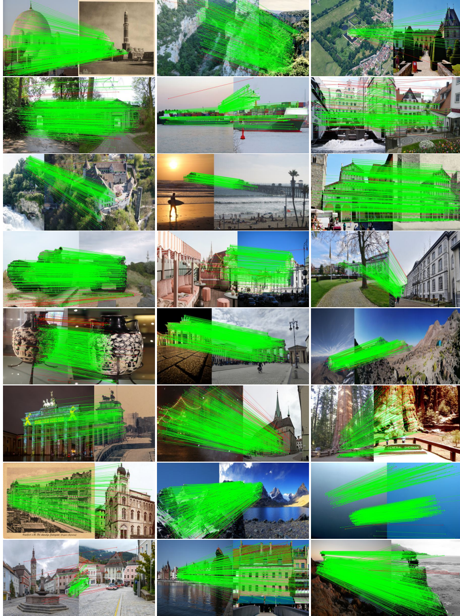
Fig. 13: LoMa-G matches from HardMatch. Inliers at 5px threshold for MAGSAC [6,7] colored green while outliers are colored red.
